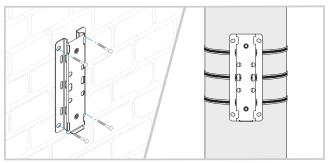
Connect bracket to wall with parapet bolts (not provided); connect to pole with band clamps (provided).
