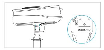
6 Attach the camera to the mounting plate using the 2 screws located on the bottom of the camera. Ensure the arrow on the plate and the camera are facing same direction.
