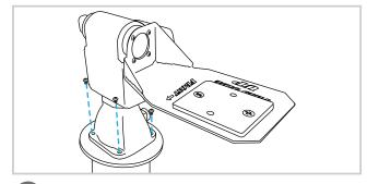
Attach the Pan-Tilt Unit to the top of the pedestal mount using the 4 sets of nuts, bolts and washers.
