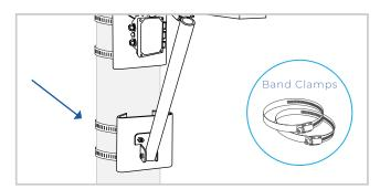
3 Attach the opposite end to the pole with 2 band clamps (provided). The support strut should be installed at a **45 degree angle**.
