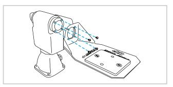
Attach the camera mounting plate to the Pan-Tilt-Unit with 4 screws.
