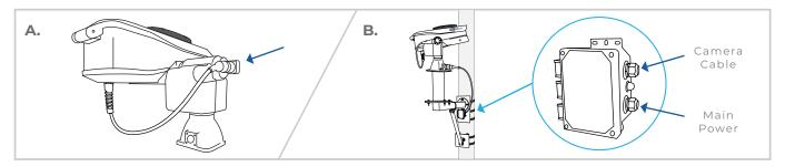
**A.** Attach the camera cable to the top connector of the Pan-Tilt Unit. **B.** Attach the Pan-Tilt Unit to the camera cable connector of the power box then attach the main power connector to the source of power, ensuring the cable is clear of being tangled. The blue light on the power box will come on and the PTU system will begin movement shortly after being powered on.
