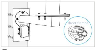
Attach the mounting arm to the pole using 3 band clamps (provided).
