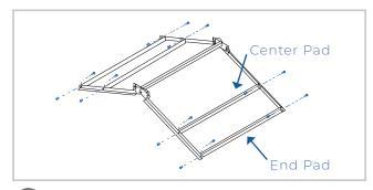
2 Attach the center pads and end pads to the left and right arms with hardware A, C, and D shown on the hardware list.
