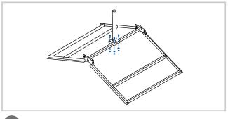
3 Attach the mast to the cross arm with hardware **F, H, and I** shown on the hardware list.
