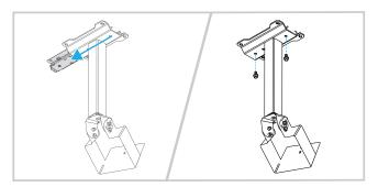
Slide universal mount onto bracket and secure with bolts (provided).
