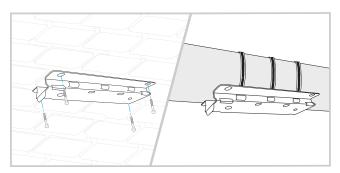
Connect bracket to wall with bolts (not provided); connect to pole or parapet with band clamps (provided).
