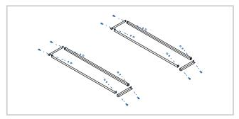
Assemble the two ballast trays using four sets of hardware A, C, D listed on page one.
