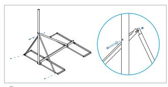
Attach the rear braces to the mast using hardware B, E, and F. Attach the other end of each rear brace to the support tube using a A, C, and D.
