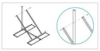
Attach the side braces to the mast using hardware B, E, and F. Connect the other end of each side brace to the ballast tray using hardware A, C, and D.
