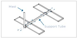
Attach the support tube and mast to the ballast trays using four sets of A, C, D. The mast is attached at the front end using the same sets of hardware.
