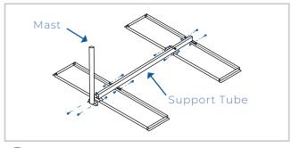
Attach the support tube and mast to the ballast trays using four sets of A, C, D. The mast is attached at the front end using the same sets of hardware.
