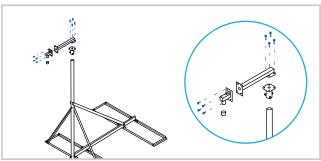
Clamp the camera arm adapter sleeve to the mast with six set screws. The camera arm assembly will ship as an assembled sub assembly.
