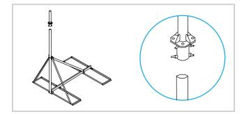
Slide the pre-assmbled mast extension over the top of the mast and lock down using the six set screws. The screws act as a leveling mechanism as well.
