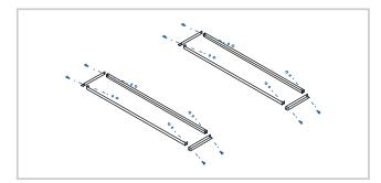
Assemble the two ballast trays using hardware four A, C, D listed on page one.
