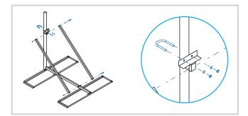
3 Attach the rear braces to the support tube using B, C, D. Loosely attach the rear braces to the clamp assembly using B, F, and C, then attach the clamp assembly to the mast.
