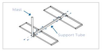
2 Attach the support tube and mast to the ballast trays using four sets of A, C, D. The mast is attached at the front end using the same set of hardware.
