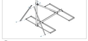
4 Attach the slotted ends of the side braces to the clamp assembly using A and E for each brace. atach the other end of each sidebrace to the ballast tray using a A, C, D.
