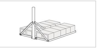
Secure the NPRM in place with 10 cinder blocks to ensure the mast is sturdy and wind resistent.
