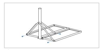
2 Attach the right and left brace angles (23" long) and the rear brace angle (28.25" long) to the frame with the following hardware - 3/8" x 1" bolt GR.5 (5), 3/8" Nut (5), 3/8" split-lockwasher (5).
