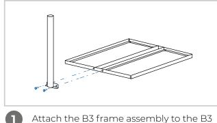
Attach the B3 frame assembly to the B3 mast assembly.
