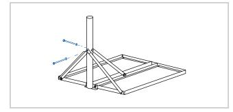
3 Attach the right, left, and rear brace angles to the mast with the following hardware - 3/8" x 4" tap bolt GR.5 (2), 3/8" USS flatwasher (2).
