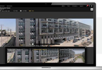
When not streaming live, the dome model can be set to take photos of 4 different camera angles every 10 minutes. This provides an expansive panoramic image and time-lapse that covers a wider project view.
